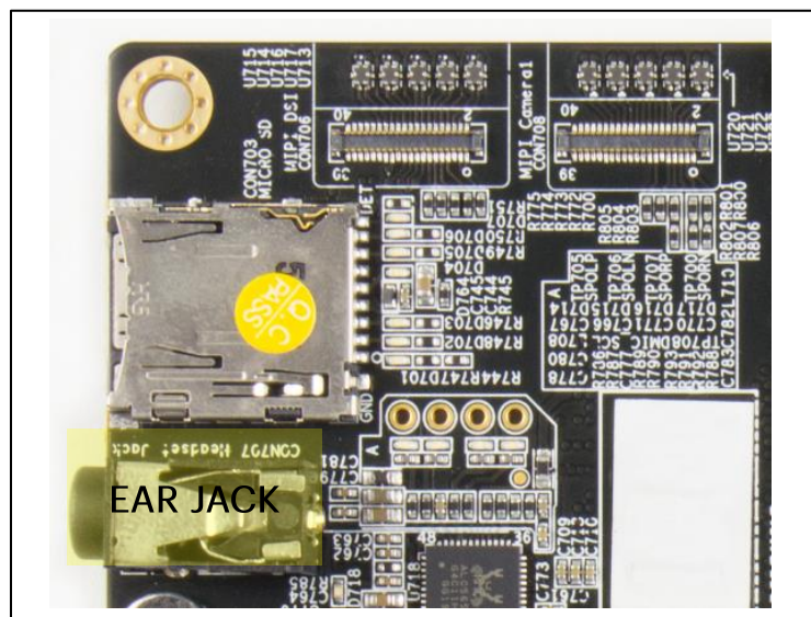
Figure 15. Ear Jack Interface location on the Platform Board
