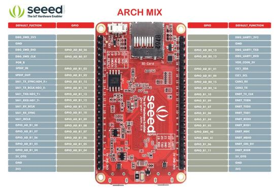
**Figure 3**. Pinout, ckick the image to view the original file
