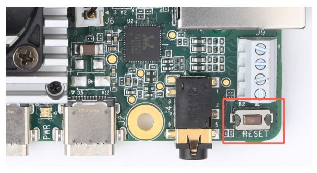
Figure 8. System reset button
