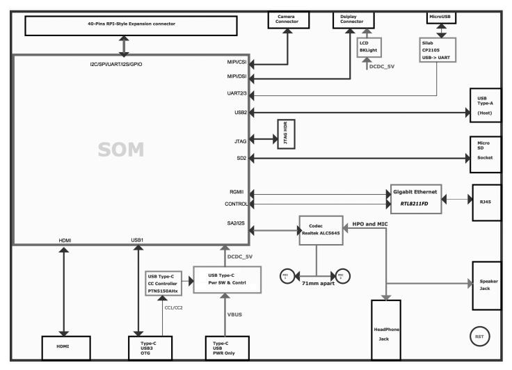
Figure 1. Block diagram of the baseboard components
