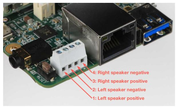
Figure 5. Stereo speaker terminals
