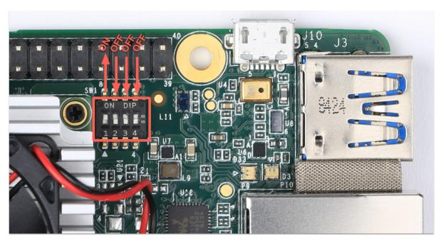
Figure 7. Boot mode switches, set to boot from eMMC
