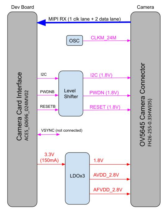
Figure 6. Camera adapter card diagram
