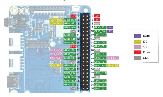
ODYSSEY - STM32MP157C's 40-pins are fully compatible with Raspberry Pi's 40-pins including GPIO, I2C, UART, SPI, I2S and PWM pins.
