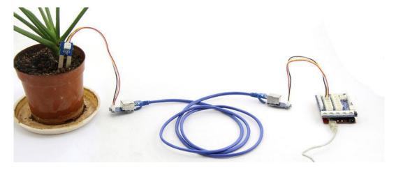
You may need to write the code by yourself for the special applications. But we can guarantee that you can always know the soil moisture of plants by observing the output data of the moisture sensor. You may want to ask why not use a long Grove cable instead of two Grove - RJ45 and a network cable, the reason is the network cable has a weak attenuation.
