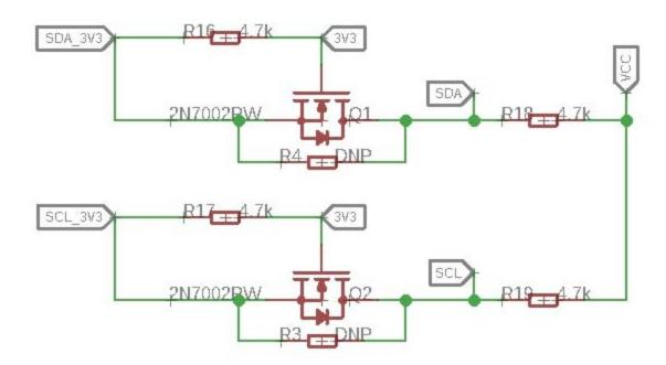
This is a typical Bi-directional level shifter circuit to connect two different voltage section of an  $I^2C$  bus. The  $I^2C$  bus of Raspberry Pi uses 3.3V, however the chip DS1307 works at 5V, so this circuit will be needed. In the schematic above, **Q1** and **Q2** are N-Channel MOSFET 2N7002A, which act as a bidirectional switch. In order to better understand this part, you can refer to the AN10441
