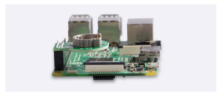
Please make sure plug the pin 1 of this hat into the pin 1 of raspberry GPIO, just like the picture above.
