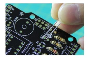
Just like the resistors, the thermistor and light dependent resistor are not polarized so it doesn't matter which way they are inserted, simply insert both leads into the board.
