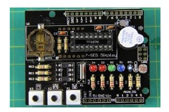
Now flip it over and finish soldering. Soldering should be second nature to you now. Notice again the desired volcano shaped solder points.
