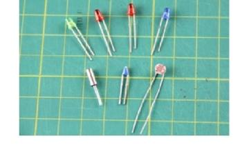
In the second row, from left to right, are a crystal, a thermistor and a light dependent resistor. They are not polarized, meaning it doesn't matter which way they are inserted into the board.
