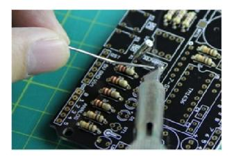
Now push down the crystal and add more solder to the locating pad. When cool, the crystal should stick to the pad.
