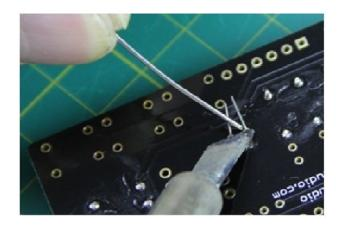
Remember the LEDs are polarized so make sure to insert them into their correct locations. The longer lead will go into hole marked "+", and place the shorter one in the other hole.
