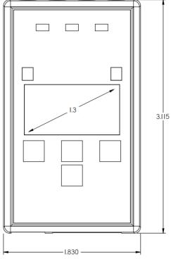
Figure 14: Xprotolab-Portable Dimensions
