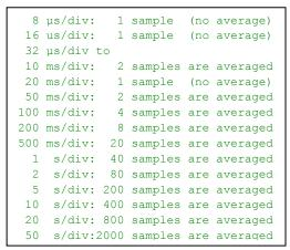
Figure 20: Number of samples averaged when enabling the channel AVERAGE option. The device's sampling rate is normally faster than needed to be able to average samples
