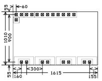
Figure 11: Xprotolab Dimensions
