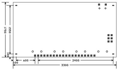
Figure 13: Xminilab 2.3 Dimensions
