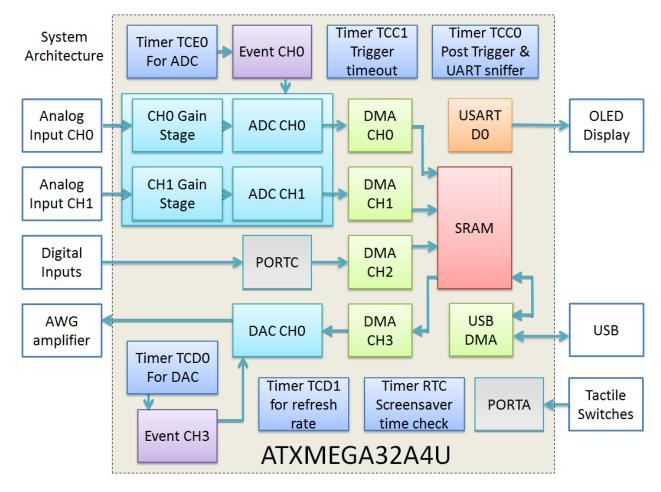
Figure 76: XScopes Architecture Block Diagram
