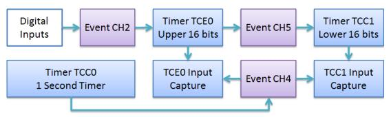
**Figure 77: Frequency Counter Block Diagram**
