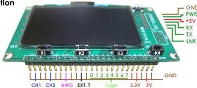
Figure 3: Xminilab HW 2.1 & 2.2 Front Signals
