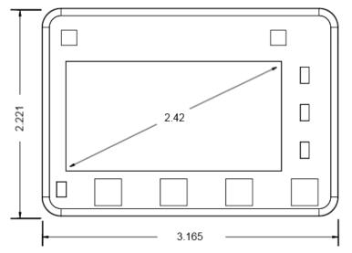
**Figure 15: Xminilab-Portable Dimensions**
