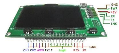
Figure 6: Xminilab HW 2.3 Front Signals
