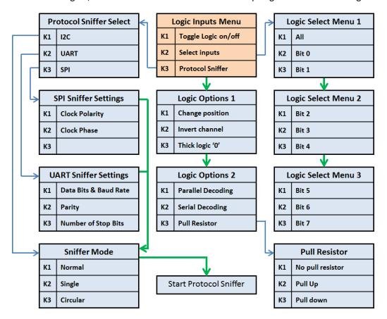
Figure 47: Logic Analyzer Menus
