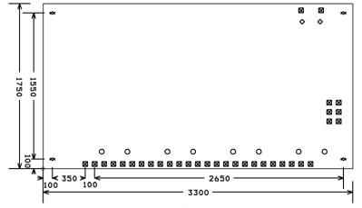
Figure 12: Xminilab 2.1 & 2.2 Dimensions
