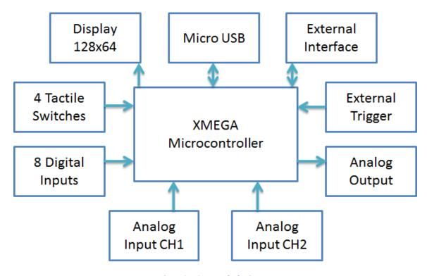
Figure 2: XScopes Block Diagram
