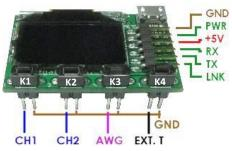
**Figure 4: Front and Top Signals**
