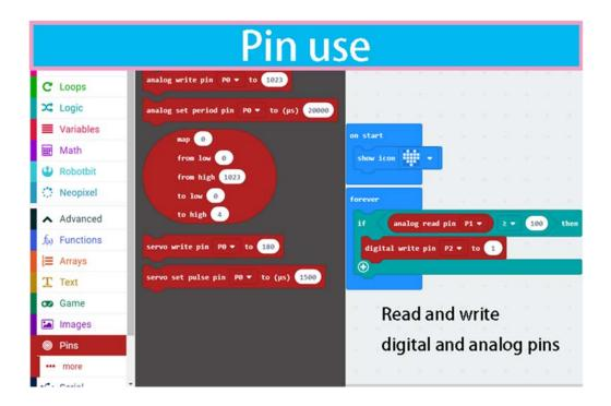
Before downloading, remember to connect to Microbit's with a micro usb cable and click the download button.
