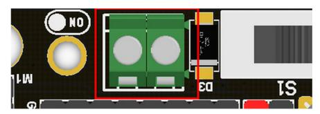
Although there is anti-reverse protection, but still pay attention while wiring. The positive and negative silkink of this interface is on the back of Robotbit. You can only input 5V or less into this port. If you have a higher voltage source you may need a LDO or DC-DC module to buck the voltage down.
