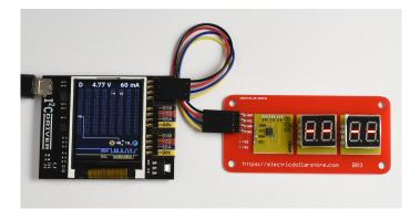
This LM75B sensor reports temperature in Celcius, so the hex byte 1A represents a temperature of 26  $^{\circ}\text{C}.$
