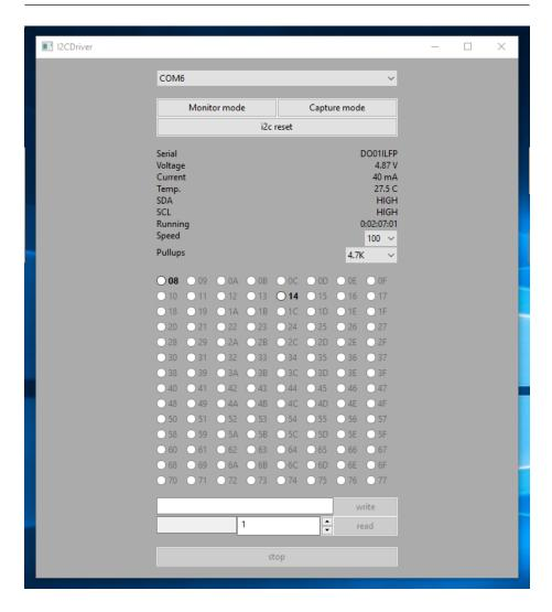
If there is only one serial device, the I<sup>2</sup>CDriver device should be automatically selected. If there is more than one device, select its COM port from the pull-down menu at the top. Once connected, you can select a connected I<sup>2</sup>C device and write and read data.
