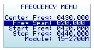
Selecting a span of 10MHz, the Start/Stop frequency changes accordingly:
