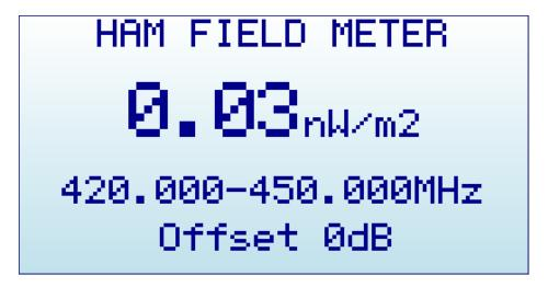
Measurement values are automatically scaled and adjusted to pico/nano/micro/milli for convenient screen reading.
