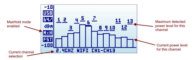
Use [RETURN] button to recycle a MaxHold capture Use [LEFT]/[RIGHT] buttons to cycle through available channels (only in 6G Combo/PLUS models)
