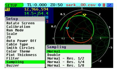
As of firmware version v0.10.17, this setup permits the following sampling modes: *«Normal»*, *«Half (Fast)» and «Double (Slow)»*. There is a separate menu to configure the resolution options.
