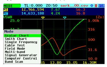
Use Navigator B to highlight the desired submenu mode option. Press the Select [ ] button to validate the selection. Press any other button to cancel the operation.
