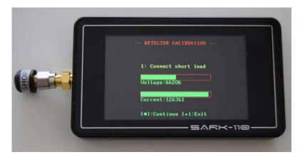
Before performing this operation, it is strongly recommended that the file containing the factory results, **detcalib.dat**, is backed up to enable a restore, if needed.
