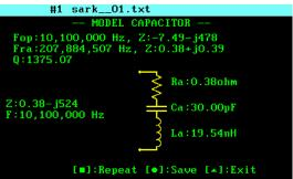
The figure below describes the measured parameters:
