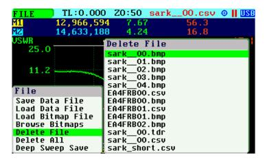
As of firmware version v0.10.18, the Delete File function was modified to allow the selection of multiple files. Use Navigator B to highlight a file to be deleted, press the Run/Hold [▶ | ] button for marking the file and iterate for all desired files. Press the Select [■] button to validate the selection. Press any other button to cancel the operation.
