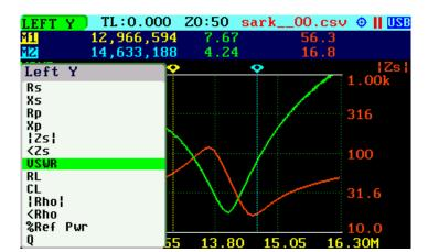
(ii) Use Navigator B when either the **«LEFT Y»** or **«RIGHT Y»** option is highlighted. Options are selected sequentially.
