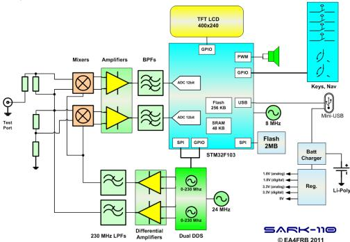
The SARK-110 comprises four main sections: a signal generator used as an active source, a bridge to provide signal separation, two tuned receivers that down convert and detect the signals and a microcontroller and display for calculating and reviewing the results.
