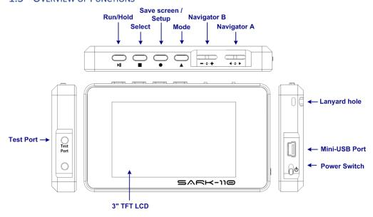
The unit has a Test Port located on its left side, to connect to the device under test. This receptacle accepts straight MCX plug connector types. The product pack includes an MCX to SMA female connector adapter and a 20-cm SMA plug to SMA female cable adapter.
