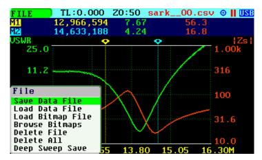
After selecting the *«Save Data File»* submenu option, enter the file name. By default, the file name has the format "sark\_\_xx.csv" (or "sark\_\_xx.tdr" for Cable Test mode), where xx is an automatically assigned number. To change the file name, use Navigator B to change the character value and Navigator A to change the character position highlighted in inverse video. Press the Select [■] button to validate the selection. Press any other button to cancel the operation.
