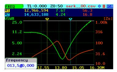
(ii) Use Navigator A to select **«FREQ»** in the main menu. Then use Navigator B to change the frequency. The frequency will change according to the current frequency multiplier. The frequency multiplier can be changed from the popup dialog, see (i) above.
