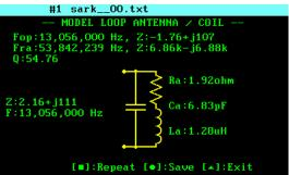
The figure below describes the measured parameters:
