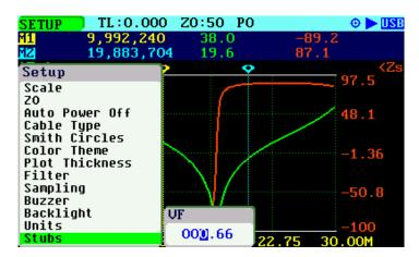
Cut a piece slightly longer than this value and connect to the analyzer. Move the Marker 1 to the point where <Zs (or Xs) crosses zero. In this case this frequency point is at 16.286 MHz
