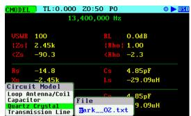
Enter the frequency value, which should be close to the expected resonant frequency of the crystal
