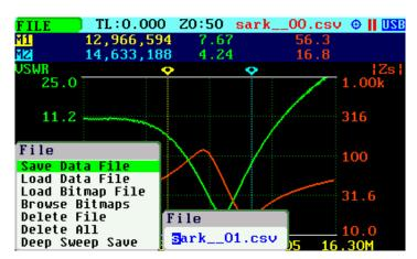
The «Save Data File» option can be also selected by pressing Navigator A when **«FILE»** is highlighted.
