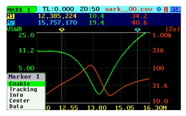
The choices are the Plot Values, Z in rectangular notation, Z in polar notation, Rho in rectangular notation or Rho in polar notation.
