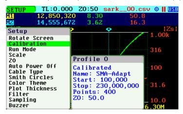
Once the calibration profile has been selected, choose **«SETUP»** *«Calibration»* «OSL» to start the OSL calibration procedure.
