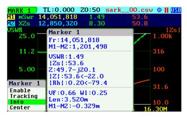
The «Center» menu option can be used to set the center frequency at the marker's frequency value.
