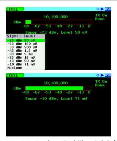
The signal generator outputs continuously unless it is on hold by pressing the Run/Hold [ | | | | button. In the Hold state the level graph and power level indicators change to red. Signal generation can be resumed at any time by pressing the Run/Hold [ > | | ] button again.
