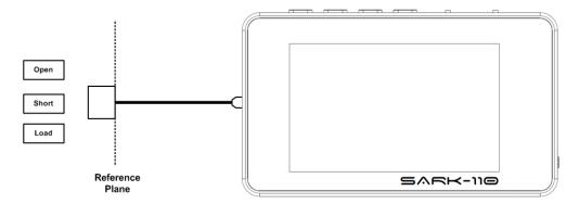
The analyzer performs a series of measurements with these loads, calculating error coefficients that are stored in a file that is automatically loaded each time the analyzer is run. These error coefficients are used to correct the measured values. The number of calibration points is fixed to 400.
