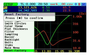
The internal disk drive can be optionally formatted. Press the Select [ ] button to format the disk or any other button if only a reset to factory defaults is required.
