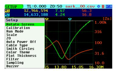
Use Navigator B to highlight the desired submenu setup option. Press the Select [ ] button to validate the selection. Press any other button to cancel the operation.
