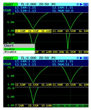
The *«Save Data File»* function operates in the same way as in other modes. The data for each band of the enabled charts is stored sequentially in individual files. The *«Load Data File»* loads the data from a file to the selected band only.
