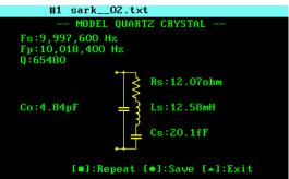
The figure below describes the measured parameters:
