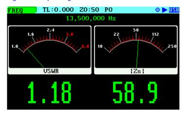
As of firmware version v0.10.4, Single Frequency mode allows taking measurements at specified time intervals that are recorded sequentially in a text file. This feature is designed for scenarios where it is necessary analyzing variations in measurements over time.
