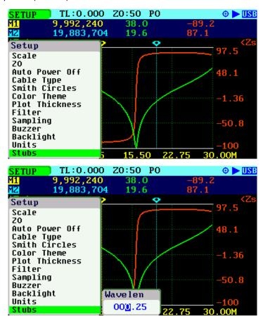
From the Scalar Chart mode, select start frequency of 1 MHz and stop frequency above the desired frequency –in this case it is set to 30 MHz
