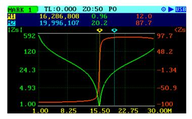
Select **«MARK 1»** *«Info»*. The readings show a length of 3.037m and a length difference (M1-M2) of 0.563m, which is the excess length of the piece of coax cable. Cut a piece slightly shorter than this value and repeat the process until getting to the expected value.
