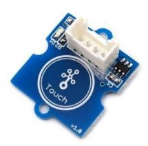
Grove - Touch Sensor enables you to replace press with touch. It can detect the change in capacitance when a finger is near by. That means no matter your finger directly touches the pad
