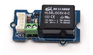
Relay is a useful tool to magnify your Arduino's control ability! Feed the control signal through the Grove interface, and relay will control the open/close of the external circuit that connected to the screw terminals. The
