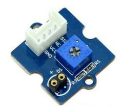
Grove - LED is designed for the beginners of Arduino/Seeeduino to monitor controls from digital ports. It can be mounted to the surface of your box or desk easily and used as pilot lamp for power or signal.
