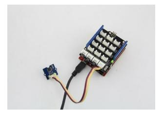
Grove – Temperature Sensor is used to detect environment temperature.
