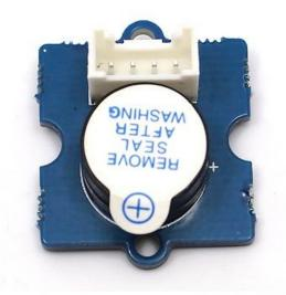
This is a simple yet enjoyable Grove to use. The piezo can be connected to digital outputs, and will emit a tone when the output is high. Alternatively it can be connected to an analog pulse-width modulation output to generate various tones and effects.
