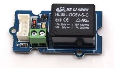
Relay is a useful tool to magnify your Arduino' s control ability! Feed the control signal through the Grove interface, and relay will control the open/close of the external circuit that connected to the screw terminals. The voltage of the external circuit can run up to 220V! So grab this relay and start
