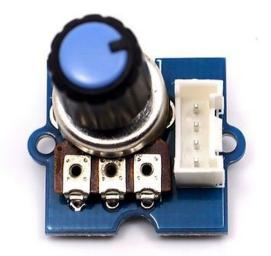
The potentiometer Grove produces analog output between 0 and VCC. The angular range is 300 degrees with a linear change in value. The resistance value is 10k ohms, perfect for Arduino use.
