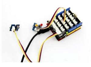
The output of the analog light sensor ranges from 0 to 1023, but the output is not linear with respect to the ambient light intensity.
