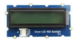
This Grove enables you to set the color to whatever you like via the simple and concise Grove interface. It takes I2C as communication method with your microcontroller. So number of pins required for data exchange and backlight control shrinks from ~10 to 2, relieving IOs for other
