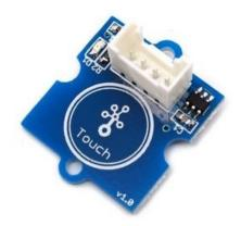
Grove - Touch Sensor enables you to replace press with touch. It can detect the change in capacitance when a finger is nearby. That means no matter your finger directly touches the pad or
