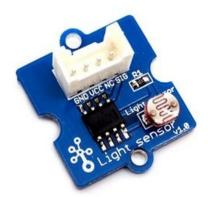
The light sensor, also known as the light dependent resistor (LDR). Typically, the resistance of the light sensor will decrease when the ambient light intensity increases.
