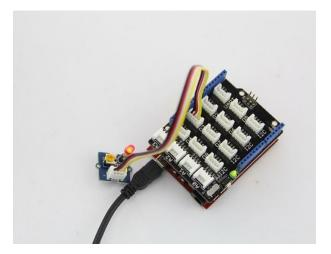
We prepare three colors of LED bulbs for you, you can get the color you want by changing the LED on the tiny Grove – LED Socket .LEDs have an cathode on the flat side of the bulb, and a anode on the round side of the bulb. The anode needs to be installed corresponding to the '+' sign on the seat for the LED to work properly.
