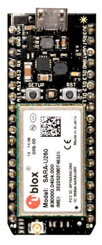
The Electron has a footprint, which is a drop-in compatible with the Particle Photon or Core.
