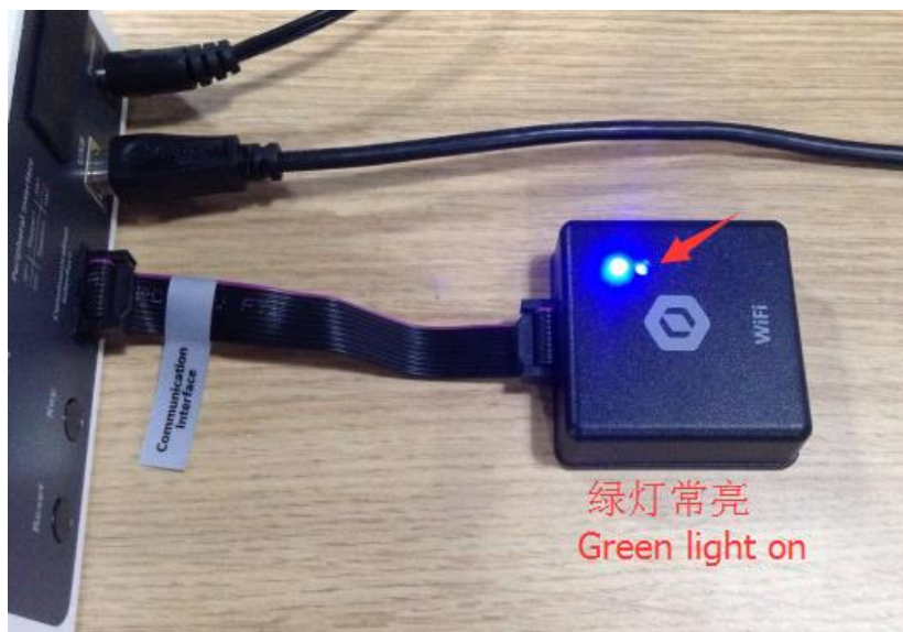
Figure 11.3 Connected with WLAN
