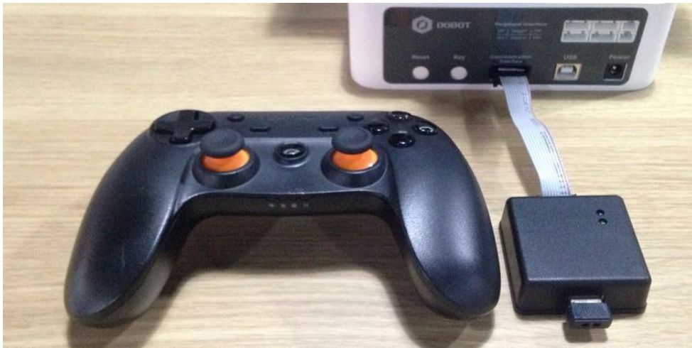
Figure 12.1 Installation of stick module
