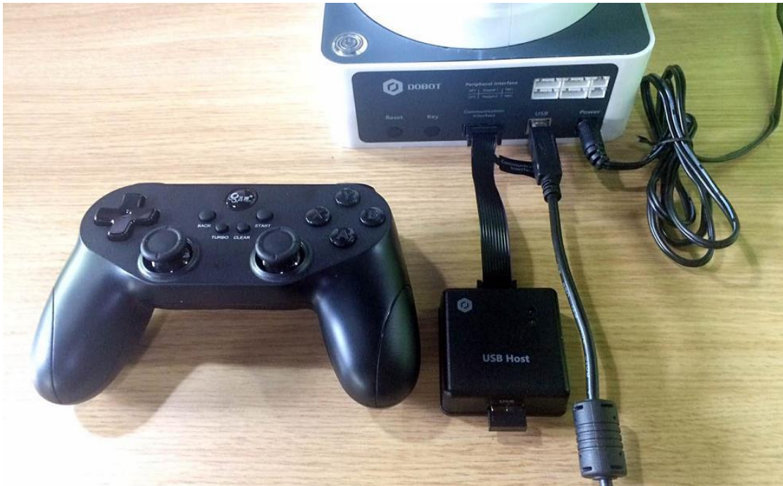
Figure 12.5 Installation of Beitong Joystick
