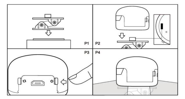
To mount MU on a toy, use the included double-sided tape. First, secure the mount on the toy. (P1)
