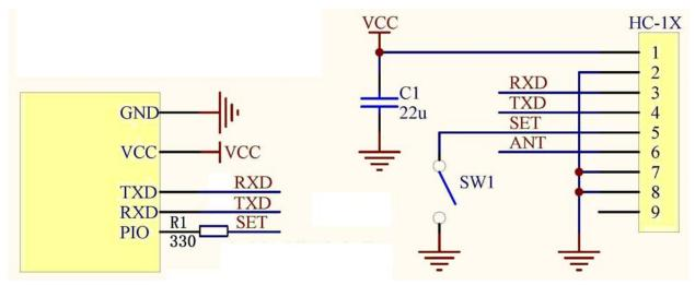
Please set the "SET" control pin to high level or hanging out in normal times, and set to low level in setting parameters state.
