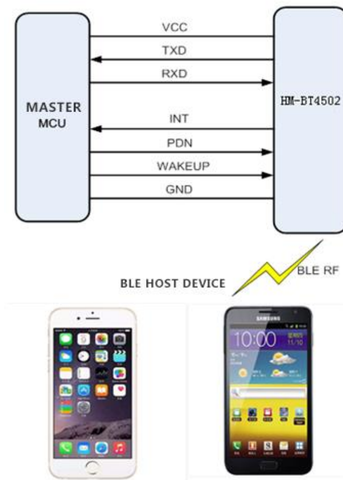
Figure 1. Application Schematic of the Pass-through Module
