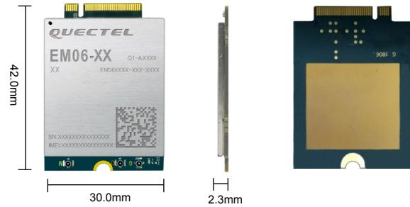
Quectel EM06 is a series of LTE Advanced category 6 module optimized specially for M2M and IoT applications. Adopting the 3GPP Rel. 11 LTE technology, it delivers maximum data rates up to 300Mbps downlink and 50Mbps uplink.
