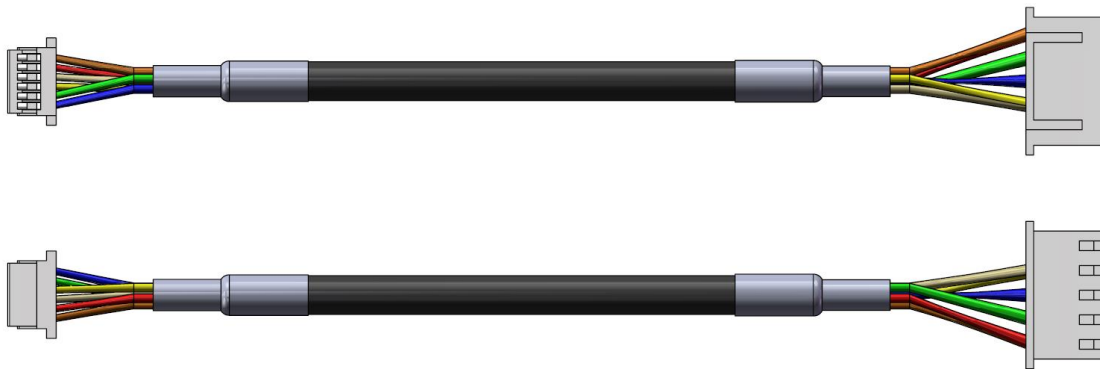
Figure 2-6 RPLIDAR S1 Interface Lead Schematic Diagram
