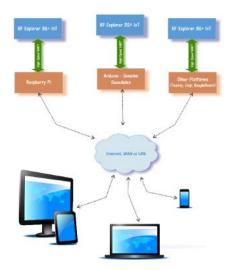
Furthermore, other platforms such as BeagleBone, Chip, Chipkit, Teensy all them can easily control a RF Explorer 3G+ IoT by manually connecting to a standard UART port.
