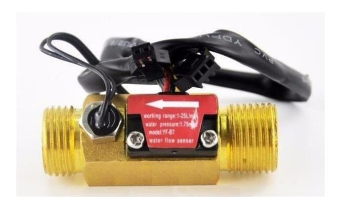
Water flow sensor consists of a copper body, a water rotor, and a hall-effect sensor. When water flows through the rotor, rotor rolls. Its speed changes with different rate of flow. The hall-effect sensor outputs the corresponding pulse signal. This one is suitable to detect flow in water dispenser or coffee machine. Life is longer than plastic body.
