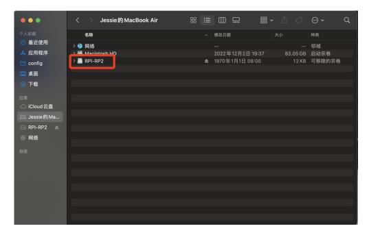
Copy the .uf2 file in the firmware package to the disk, then the disk will log out.
