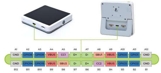
Note: A2, A3, A10, A11, B2, B3, B10, B11 connect to RP2040 GPIO8, GPIO9, GPIO0, GPIO1, GPIO2, GPIO3, GPIO15, GPIO14
