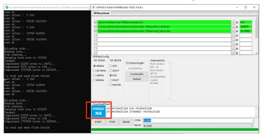
There is "indicator\_terminal\_demo.bin" firmware (allinone ) in the <u>sdk</u> . you can flash it to esp32.
