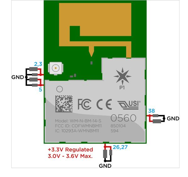
Fig. 1 Recommended power connections with decoupling capacitors.
