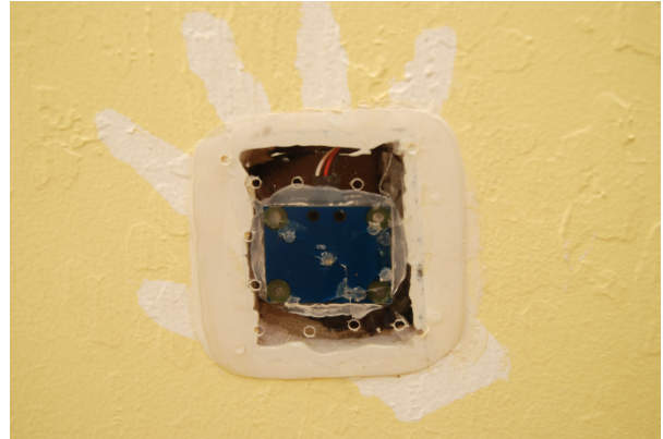
Cover hole with a thin piece of plastic/acrylic (less than 1/8" thick), glue touch sensor to plastic/acrylic piece
