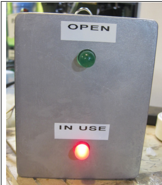
Example LED indicator box for the Photobooth. The green LED means the Photobooth is in idle mode and the red LED means the Photobooth is in use.
