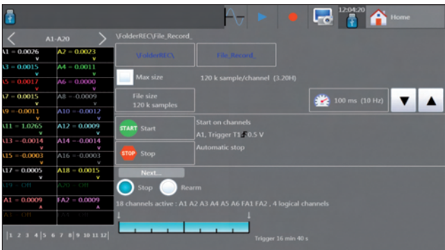
Trigger: multiple choice and combination of threshold, channels and conditions
