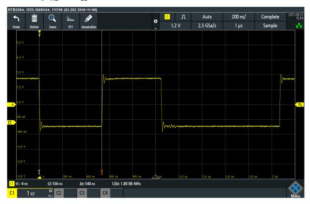
$t_{AB}$  is measured as 540ns.
