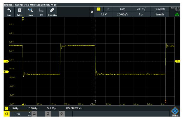
$t_{\text{CD}}$  is measured as 1020ns.
