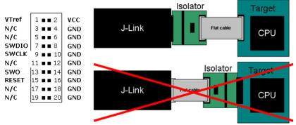
The Emulator side of the Isolator is plugged directly into the Emulator. The Target side is connected to the target via a 20-pin flat cable.
