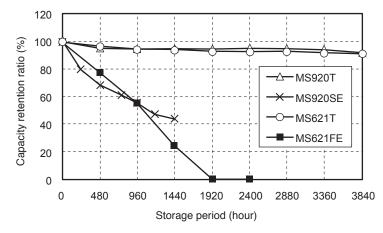
MS-T series' capacity retention ratio after High temperature storage were greatly improved. \* 85°C use of Conventional MS series is not guaranteed.
