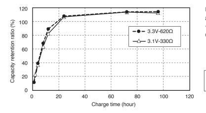
Both the MS621T and MS920T can reach 80% of capacity after 12 hours of charging. \*MS920T: Calculated given a 100% charge of 6.5 mAh nominal capacity.
