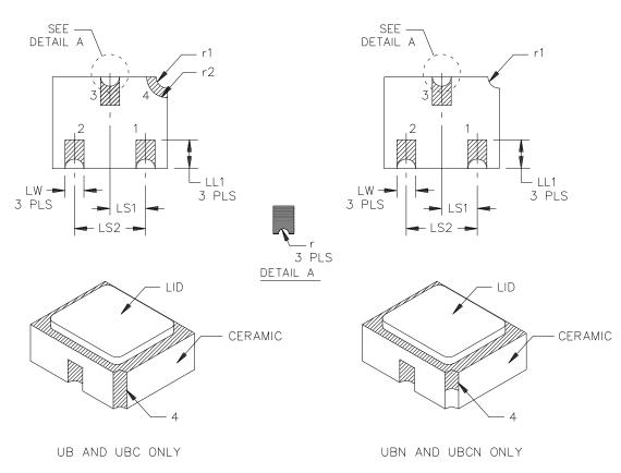
FIGURE 3. Physical dimensions, surface mount (UB, UBN, UBC, and UBCN versions).
