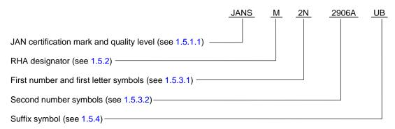
\* 6.6.2 <u>Unencapsulated devices</u>. The PINs for un-encapsulated devices are constructed using the following form.
