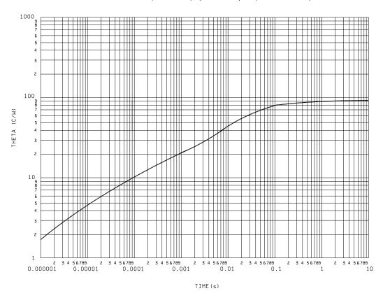
FIGURE 15. Thermal impedance graph (R<sub>θJSP(IS)</sub>) for 2N906A and 2N2907A (UB, UBC, UBN, and UBCN).
