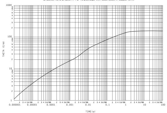
FIGURE 12. Thermal impedance graph ( $R_{\theta JC}$ ) for 2N2906A, 2N2906AL, 2N2907A, and 2N2907AL (TO-18).
