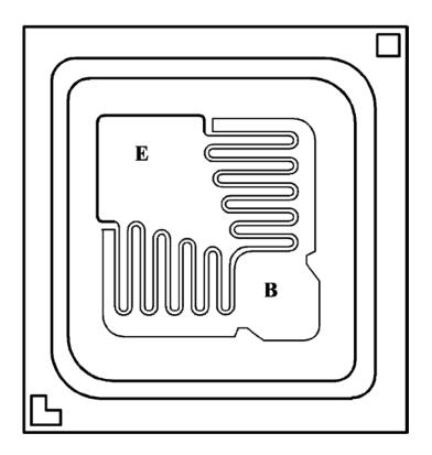
1. Chip size: .023 x .023 inch ±.002 inch (0.584 mm x 0.584 mm ±0.0508 mm).
