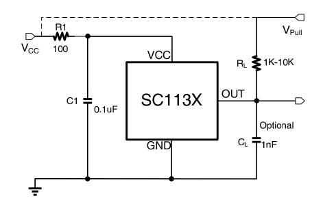
The SC113X contains an on-chip voltage regulator and can operate over a wide supply voltage range. In applications that operate the device from an unregulated power supply, transient protection must be added externally. For applications using a regulated line, EMI/RFI protection may still be required. R1 is for improved CI performance, and could be 100 or 200  $\Omega$  typically.
