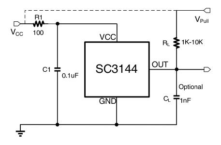
The SC3144 contains an on-chip voltage regulator and can operate over a wide supply voltage range. In applications that operate the device from an unregulated power supply, transient protection must be added externally. For applications using a regulated line, EMI/RFI protection may still be required. R1 is for improved CI performance, and could be 100 or 200  $\Omega$  typically.
