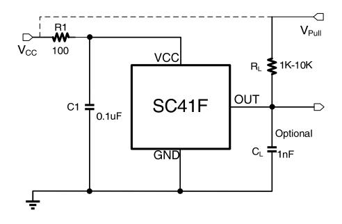
The SC41F contains an on-chip voltage regulator and can operate over a wide supply voltage range. In applications that operate the device from an unregulated power supply, transient protection must be added externally. For applications using a regulated line, EMI/RFI protection may still be required. R1 is for improved CI performance, and could be 100 or 200  $\Omega$  typically.
