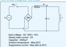
The most suitable power thermistor for the above circuit is required to fulfill the following terms and conditions.
