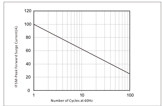
Figure 6. Maximum Non-Repetitive Forward Surge Current Uni-Directional Only
