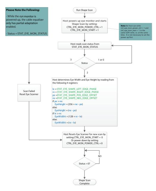
Figure 4-8: Shape-Scan Flow Diagram
