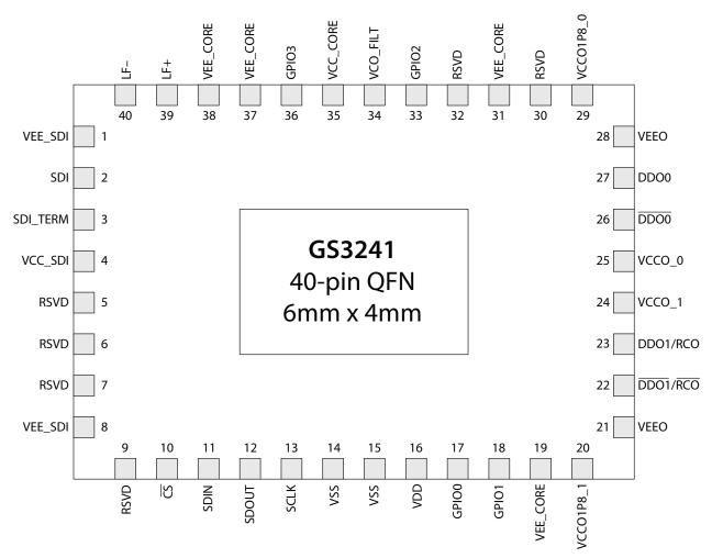
Figure 1-1: GS3241 Pin Assignment
