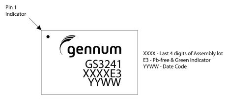
Figure 7-3: Marking Diagram
