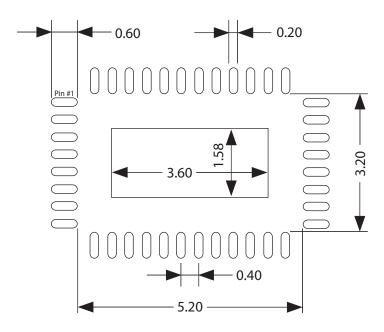
Figure 7-2: Recommended PCB Footprint
