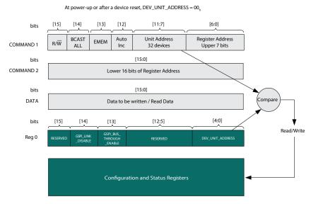
Figure 4-35: Internal Register Map Functional Block Diagram
