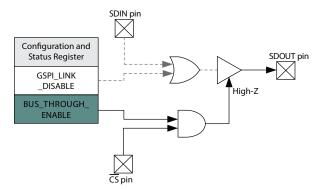
Figure 4-21: GSPI\_BUS\_THROUGH\_ENABLE Operation
