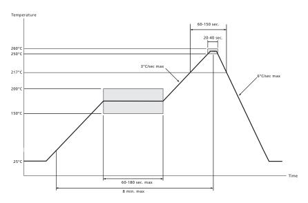
Figure 7-4: Maximum Pb-free Solder Reflow Profile
