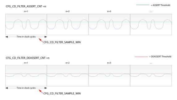
Figure 4-1: STAT\_PRI\_CD Configuration Parameters
