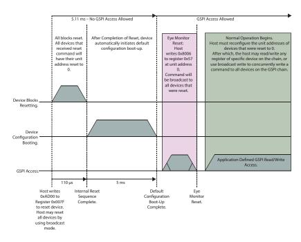
Figure 4-37: Host Initiated Device Reset Timing Sequence.
