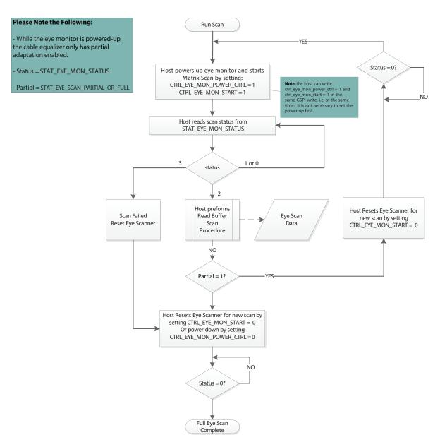
Figure 4-9: Matrix-Scan Flow Diagram
