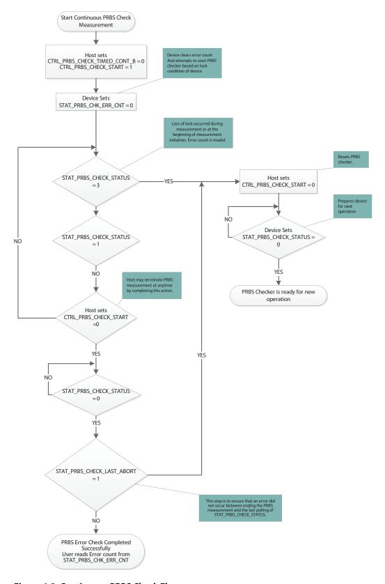
Figure 4-3: Continuous PRBS Check Flow
