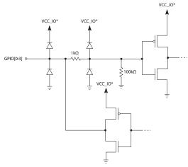
Note: VCC\_IO makes reference to the following power supplies and pins: VCC\_IO = VDD for GPIO[0:1] VCC\_IO = VCC\_CORE for GPIO[2:3]
