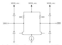
**Note:** The <n> is VCCO\_<n> refers to the output power supply number. VCCO\_1 is the power supply connection for DDO1/ $\overline{DDO1}$ , and VCCO\_0 is the power supply connection for DDO0/ $\overline{DDO0}$ .
