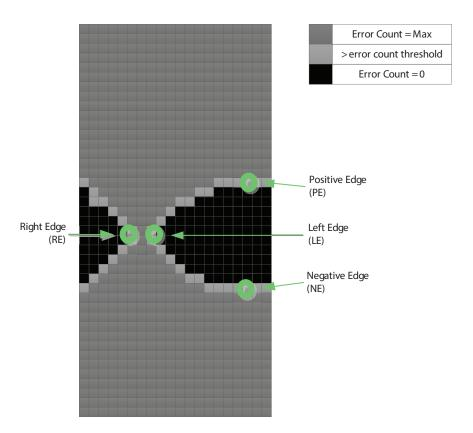
Figure 4-7: 4-Point Scan Coordinates Relative to the Eye
