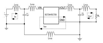
Figure 1 - PCB Circuit with Equivalent Parasitic Inductance
