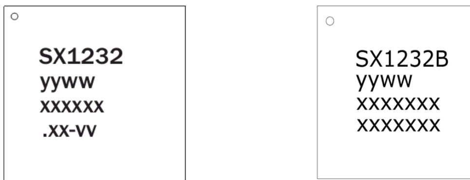
Figure 3. Marking Diagram SX1232 & SX1232B
