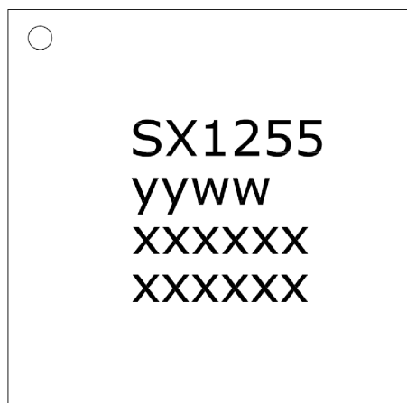
Figure 7-3: SX1255 Marking Diagram
