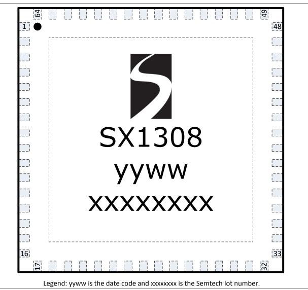
Figure 1: Top View of SX1308 Package with 64 Pins & Exposed Ground Paddle (Package Bottom)
