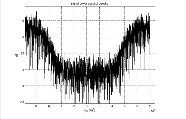
The following plot gives the spectral power content of the I/Q bit stream.
