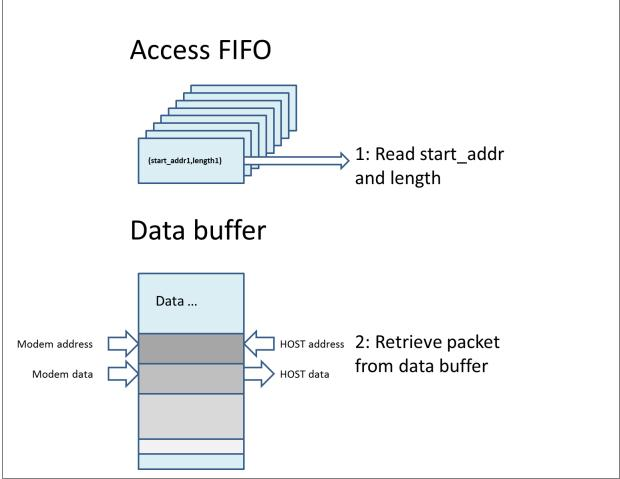
Figure 7: Access FIFO and Data Buffer
