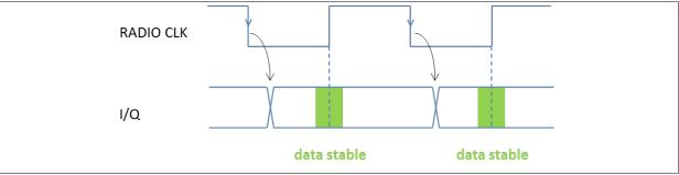
Figure 5: I/Q on Clock Falling Edge
