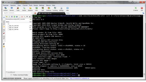
Figure 15: Load STM32F401CD MCU Binary
