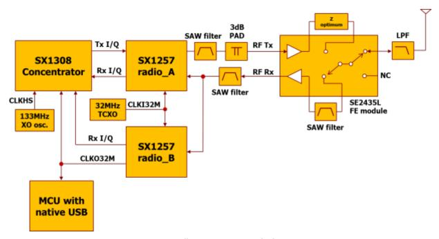
Figure 3: PicoCell Gateway V1.0 RF Block Diagram
