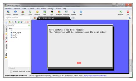
Figure 11: raspi-config "Expand Filesystem"
