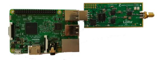
Figure 6: Raspberry Pi and PicoCell GW Connection
