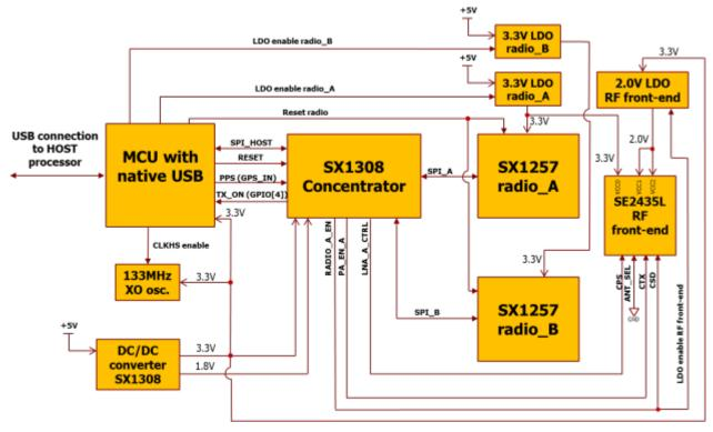
Figure 4: PicoCell GW V1.0 HW Control Signals
