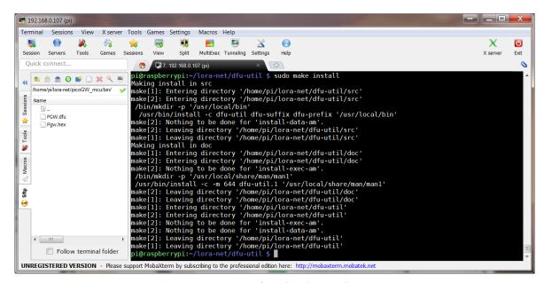
Figure 13: Dfu-util Make Install
