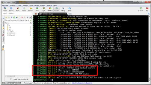
Figure 17: "dmesg" Command Result
