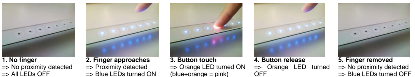
Figure 52 Touch+Proximity Module Operation
