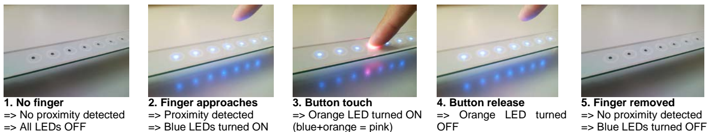
Figure 63 Touch+Proximity Module Operation
