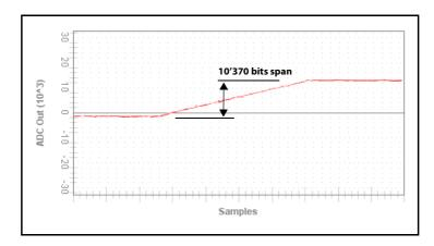
Figure 44. Signal Span Using Zooming Settings
