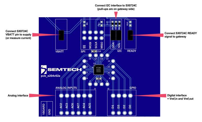
Figure 5. SX8724C Interface on the Board
