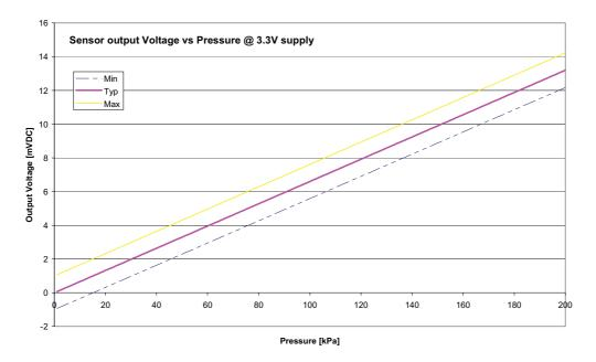
Figure 31. Sensor transfer function
