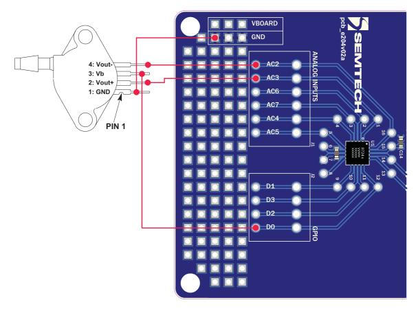
Figure 33. Connection on the SX8724CEVK Evaluation board
