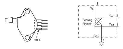
Figure 30. Pressure sensor pin out & equivalent schematic
