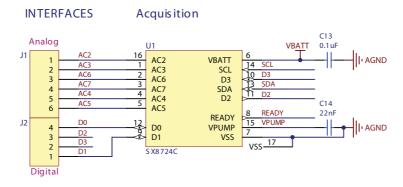
Figure 4. Analog Interface Schematic
