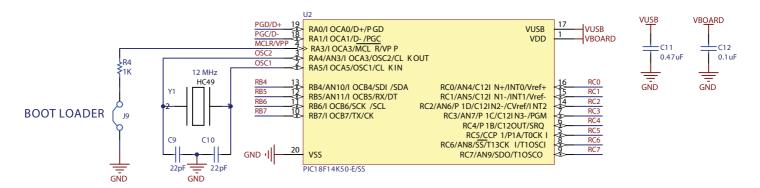
Figure 9. PIC Gateway Schematic
