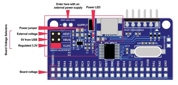
Figure 8. SX8724CEVK Power Supply Selector
