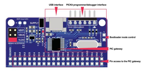
Figure 10. PIC Gateway on the Board
