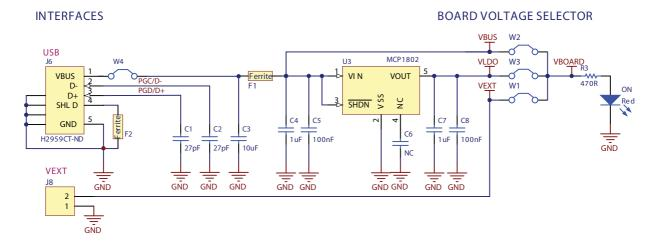
Figure 7. Power Supply Schematic
