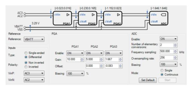
Figure 20. Zooming ADC Control Sections
