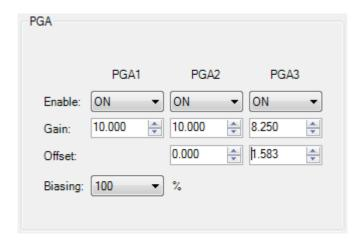
Figure 41. SX8724C "PGA" final configuration
