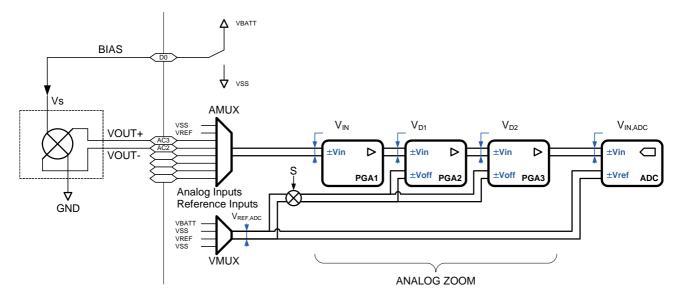
Figure 32. Sensor schematic connection to the SX8724C
