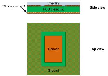
Figure 6: Typical Capacitive Sensing Implementation
