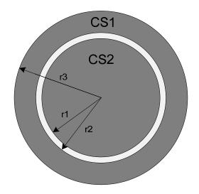
Figure 21: Typical Smart Sense Capacitive Sensor
