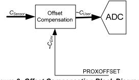
Figure 9: Offset Compensation Block Diagram
