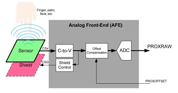
Figure 8: Analog Front-End Block Diagram
