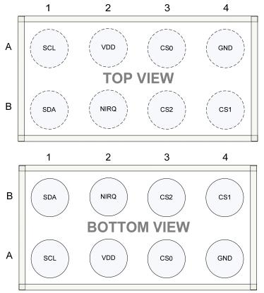
Figure 1: Pin Diagram
