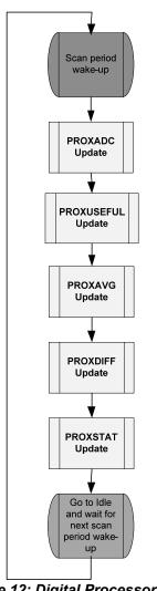
Figure 12: Digital Processor Sequence
