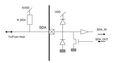
Figure 30: SDA Simplified Diagram
