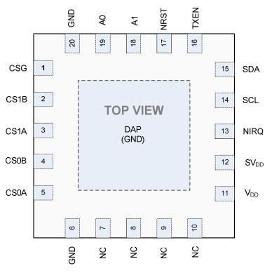
Figure 1: Pin Diagram
