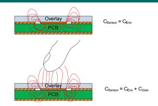
Figure 8: Proximity Effect on Electrical Field and Sensor Capacitance
