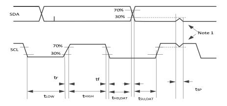
Figure 4: I2C Data Timing
