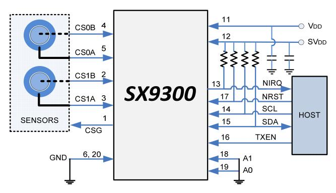
Figure 31: Typical Application Circuit
