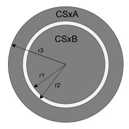
Figure 22: Typical Smart SAR Capacitive Sensor
