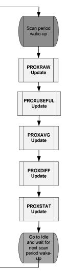
Figure 13: Digital Processing Sequencing
