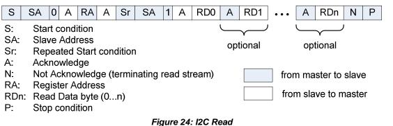
The register address is incremented automatically when successive register data (RD1...RDn) is retrieved by the master.
