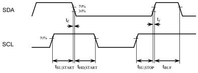
Figure 3: I2C Start and Stop Timing
