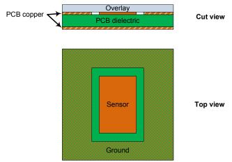
Figure 7: Typical Capacitive Sensing Implementation
