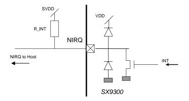
Figure 28: NIRQ Output Simplified Diagram
