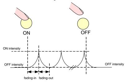
Figure 35 Continuous Fading Mode
