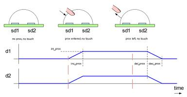
Figure 36 LEDs in triple reporting mode proximity
