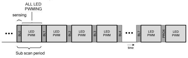
Nine (9) scan periods (1 frame) are required to scan all 8 buttons & Perform Combined Channel Proximity Sensing Figure 7 CapSense Scan Frame SX9510/11
