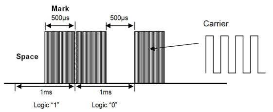
Figure 24 Phase Encoding Example (RC6) with Inverted Polarity
