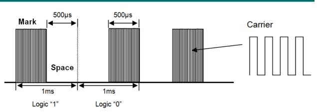
Figure 23 Phase Encoding Example (RC5) with Normal Polarity
