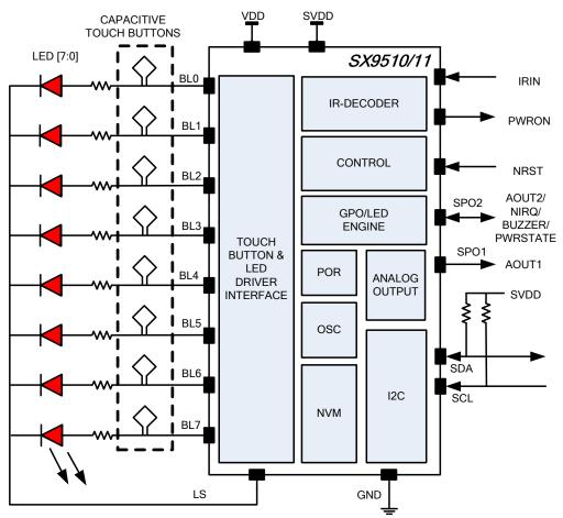
Figure 4 Simplified Block diagram of the SX9510/11
