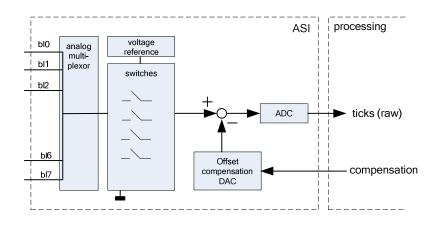
Figure 20 Analog Sensor Interface for SX9510, Combined Channel Prox Mode
