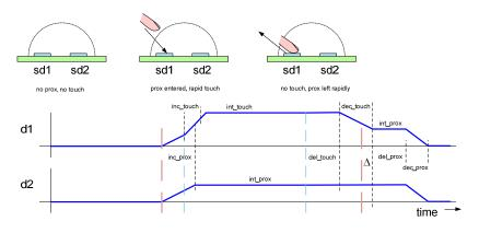
Figure 37 LEDs in triple reporting mode proximity and touch
