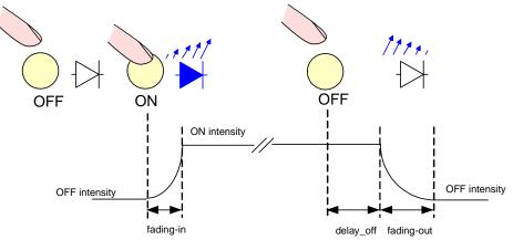
Figure 34 Single Fading Mode
