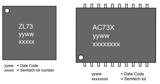
Figure 3 Marking Information SX9510 (QFN, TSSOP)
