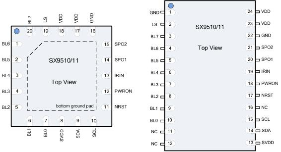
Figure 1 Pinout Diagram SX9510/11 (QFN, TSSOP)
