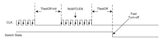
Figure 3: High-speed Turn-off Mode
