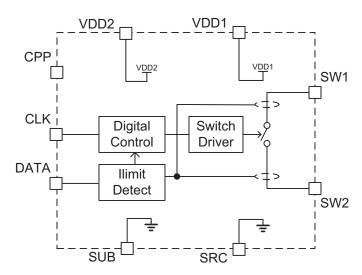
Figure 1: TS13001 Block Diagram
