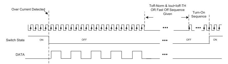
Figure 4: Over-current Shut-down and Restart
