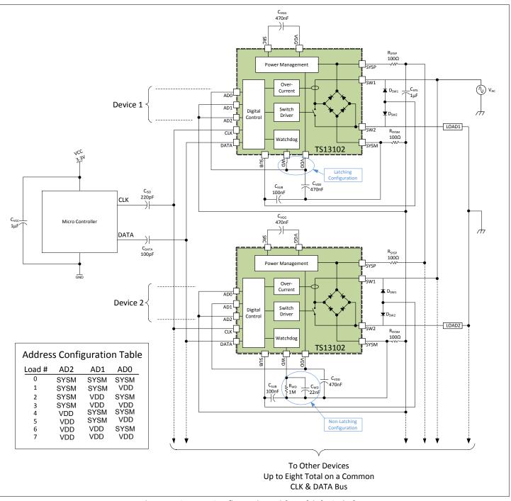
Figure 5: System Configuration with Multiple Switches
